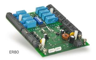
Expansion module for either processing units or attendance terminals. Expands the number of inputs and outputs and thus simplifies control. Up to 4 ER80 modules can be connected to each supervising unit expanding the number of input ports and output relays to 32 of each. These ports can be programmed separately and assigned logical functions.
