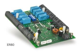
Universal module for either connection of several readers to single processing unit's port or data format conversion. Any 2 readers can be connected to inputs of the module, the output will then provide data in ACS-line formats or for processing in computer via either USB or COM port.
